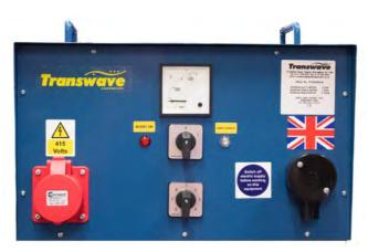
Care should be taken with the connection of the machine to the output plug/socket. If the machine has a contactor starter the 400/415v control coil must be fed from the phases marked L1, and L3. If the control circuit is fed incorrectly (i.e. connected to the phase marked L2) the contactor will either not operate or chatter when operating. Similarly, a control transformer and/or lighting transformer with a primary winding of 415v must be fed from the L1 and L3 phases.
